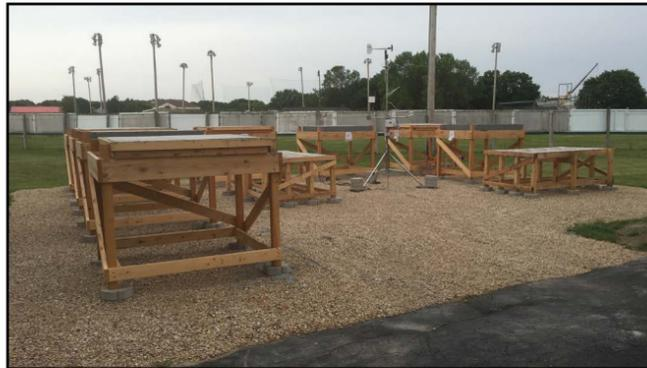
Photo 2. An overall view of the exterior slabs and smaller sample pans, exposed to the full weather, at SRI Consultants facility Wisconsin. SRI Photo
