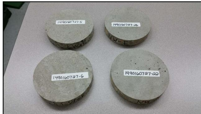
Photo 3. Specimens of the light weight structural concrete and regular weight concrete utilized to make both the slabs and specimens in Photos 1 and 2. These specimens were utilized for ASTM E96 vapor transmission testing. SRI Photo
