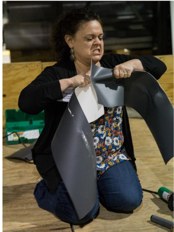
Testing a TPO weld at a hands-on training at Bone Roofing Supply (CRCA Photo)
